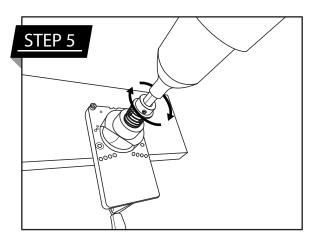
**Drill the Hinge Hole** Drill the hinge cup hole carefully into the material using the Forstner drill bit.
