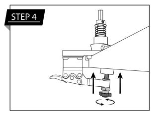
**Adjust Offset & Secure Jig** Set the offset (default 5mm) by moving the knurled nuts. Locate & secure the jig by adjusting the rubber foot.
