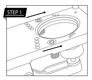
**Set 0 mark** Secure the knurled nuts to the two #20 thread positions (marked as "0").
