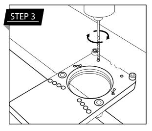
**Drill the Screw Holes** Drill two screw holes, 37mm from the material edge & spaced 32mm apart.
