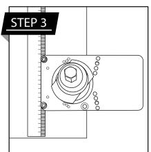
**Drill Consistent Holes** Drill hinge holes in consistent locations, using the ruler as a reference.
