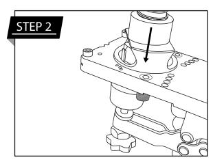
**Setup Offset** Move the bottom knurled nuts into the #20 locator position under the jig.
