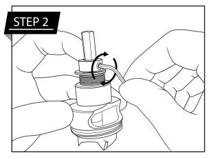
**Set the Depth** Adjust the drill bit depth to match your hinge depth, lock the stop collar in place with the spring compressed.
