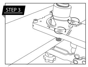
**Position the Jig** Place the jig firmly against the edge of your material for proper alignment.
