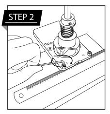
Assemble the Drill Guide Insert the Forstner drill bit to the drill guide and loosely add the spring, washer, and locking nut.
