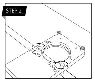
**Position the Jig** Clamp the hinge jig tight against the material edge for accurate alignment.
