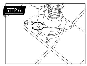
**Drill Screw Holes** Drill the screw holes according to the dimensions of your hinge.
