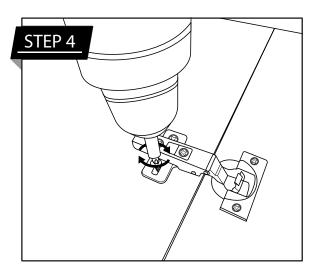
**Install the hinge** Position the hinge mounting plate and secure with screws, ensuring perfect alignment.
