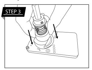
**Insert the Drill Guide** Screw the drill guide into place on the locator plate, ensuring it's tight and aligned.
