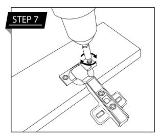
**Install the Hinges** Insert the hinge into the cup and secure with screws, ensuring perfect alignment.
