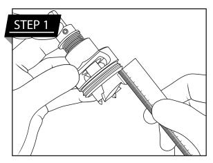
**Assemble the Drill Guide** Insert the Forstner drill bit to the drill guide and loosely add the spring, washer, and locking nut.
